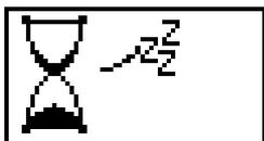
**Standby time:** the standby time in seconds indicates the time period after which the display turns off to extend the service life of the lighting cathode. The apparatus only switches to standby mode if it is flushed and if it is in main menu mode (all valves closed).
