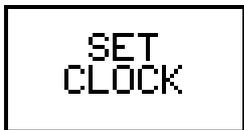
**Time:** press the [SET CLOCK] key in order to set the internal clock of the apparatus. The clock has a power reserve of approximately 10-14 days. The clock is necessary to print logs and for storing alarm messages.
